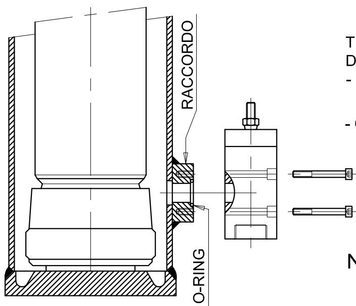
THE VALVE MUST BE INSTALLED DIRECTLY ON THE RAM WITH:
